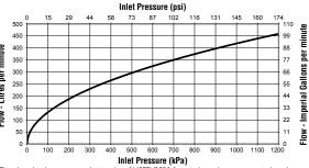
This chart has been prepared using the of HSFPV2520 from independent tests carried out by The University of Auckland, New Zealand.
