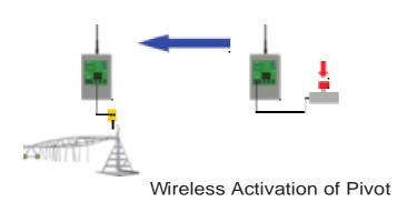
Wireless remote control of pumps and valves that can be achieved automatically using an irrigation controller or manually using a simple switch. Up to two pumps / valves can be remotely controlled from the same transmitter module. Up to two pumps / valves can also be controlled from a common receiver module or split between two receiver modules.
