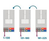
Each A2C-D75 decoder output module enables 75 stations, and allows up to three two-wire paths to the field. You can easily connect more than 75 stations to a single wire path, by assigning stations from one module to another.
