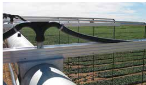
Sprinkler height can be varied by drop hose length.
