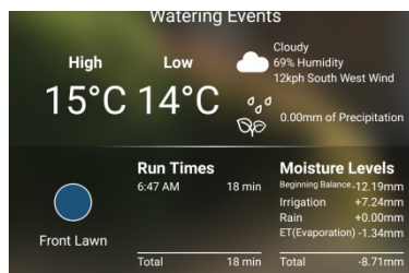
Result of irrigation showing; starting moisture level + irrigation - rain fall - evaporation = net moisture in root zone
